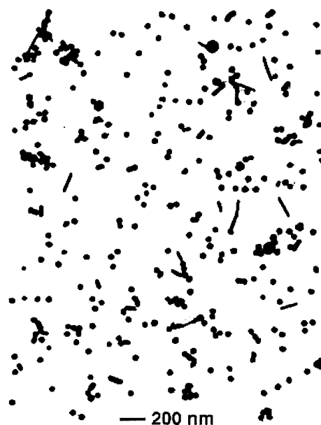
Figure 5. Representative TEM image of enlarged colloidal Au particles prepared by a two-step NH 2 OH seeding of colloidal Au (0.05 mL of 16.8 nM, 12-nm-diameter colloidal Au added to an unstirred mixture of 2.4 mL of 0.01%HAuCl 4 /0.1 mL of 40 mM NH 2 OH, then 0.1 mL of 1% HAuCl 4 added after \sim 2 min).
